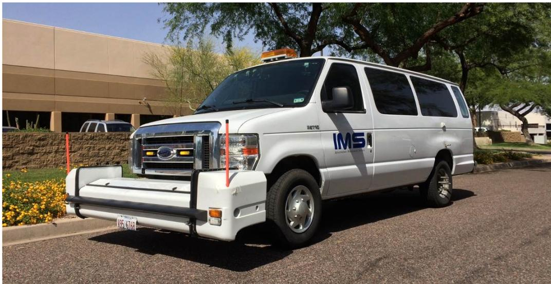
**Figure 5 – Laser Road Surface Tester (Laser RST)**
