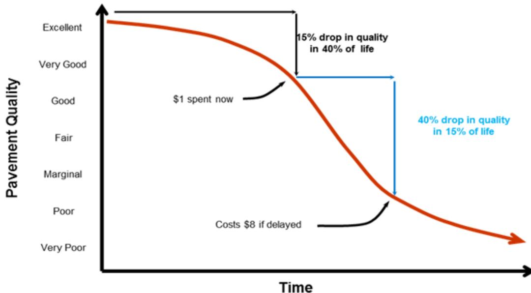
**Figure 2 – Pavement Deterioration and Life Cycle Costs**
