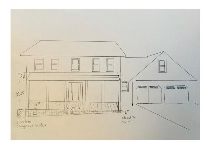
Elevation on Southside closest to creek will be 2' and elevation on Northside will be 6'' due to slope.
