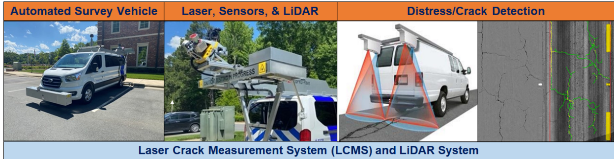
Figure 1. Laser Crack Measurement System for pavement condition assessment.
