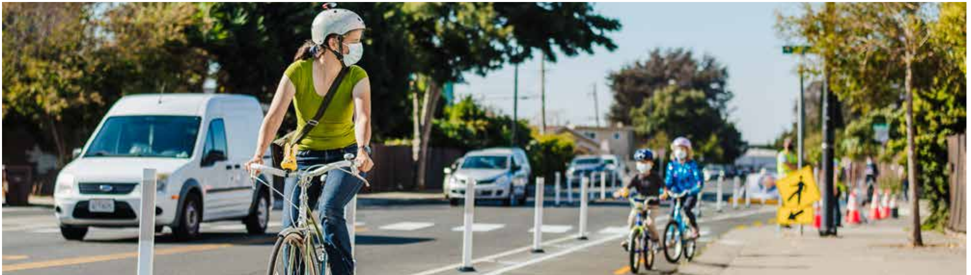
Two-way, quick build cycle track in San Pablo, CA. Source: Toole Design Group
