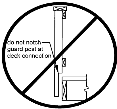
FIGURE 28: NOTCHING AT GUARD POSTS
